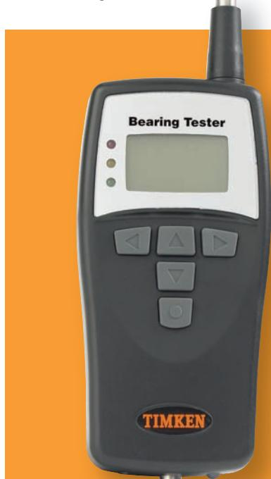
Timken's bearing tester is a portable, pocket-sized condition monitoring instrument. It is reliable, affordable and easy to use. The compact and lightweight design make the bearing tester a convenient tool for assessing the health and lubrication condition of ball- and roller-type bearings in many industrial environments.
