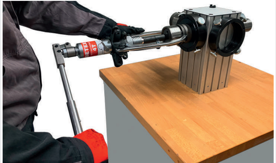
14 Use of the hydraulic puller HSP
