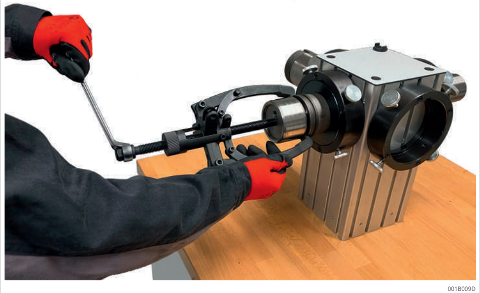
2 Use of the mechanical puller MSP-2/3
