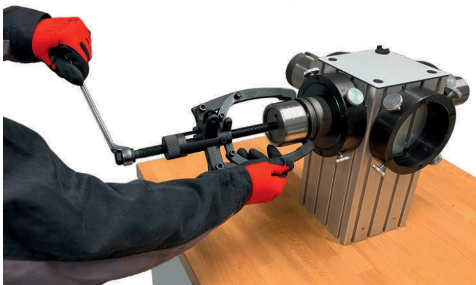
10 Use of the mechanical puller MSP-2/3
