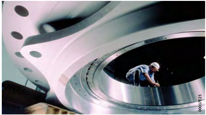
Figure 1 Double row FAG spherical roller bearing in the London Eye
