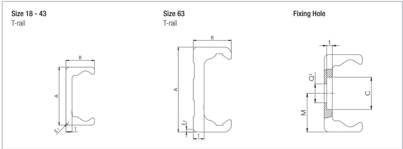
Q<sub>1</sub> Fixing holes for Torx® screws with low head (custom design) included in scope of supply
