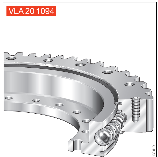
Figure 1 · Designation – example of four point contact bearing
