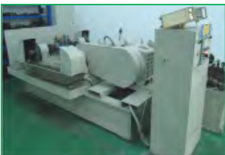
Test di usura Chain wear testing machine
