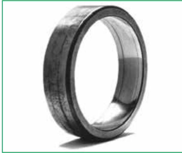
Fig. 16 Full running path pattern around entire raceway circumference of stationary outer ring of self-aligning ball bearing with rotating inner ring
