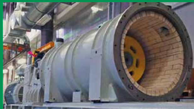
Above the ISB SNL bearing unit. On the left an industrial mill
