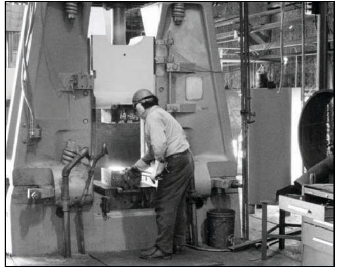
One of the many hammers capable of producing forgings up to 50 lbs.
