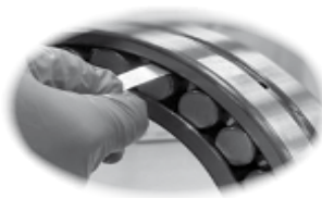
Measure of RIC before installation
