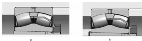
Adapter sleeve mounting without additional axial support
