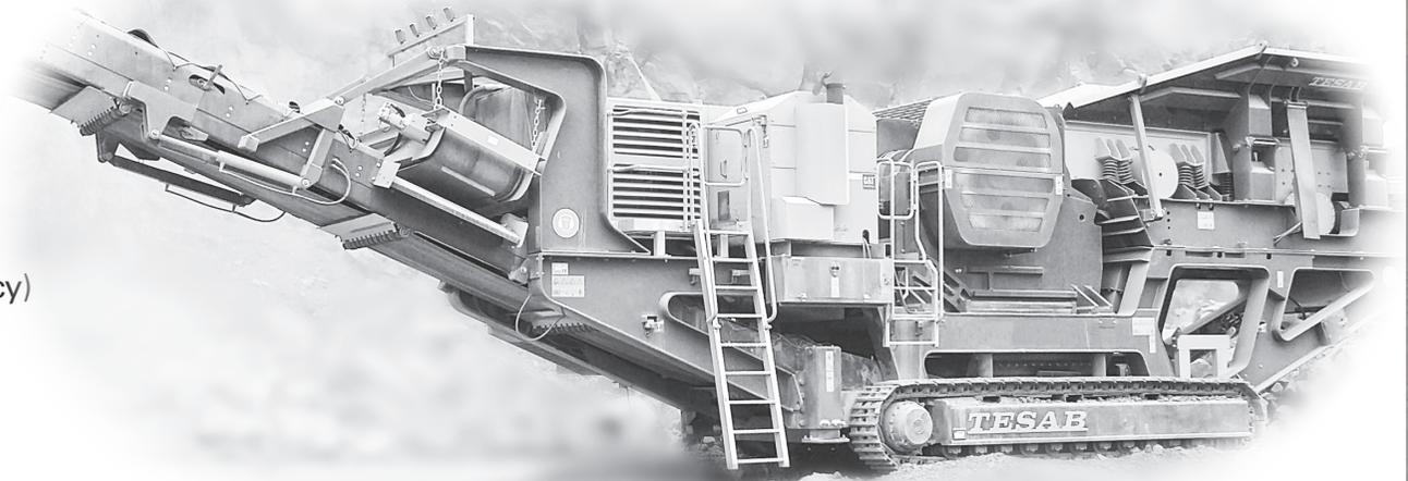
Providing correct bearing support for screen excitation mechanism is one of the most challenging tasks for screen designers and bearing providers. Bearings must be able to tolerate the misalignment created by shaft bending and frame deflections, to cope satisfactory with intense rotating acceleration fields generated by the vibrating motions, to accommodate shaft thermal expansion, and to support the dynamic loads from the eccentric movement as well as the shock loads from material processing.
