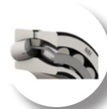
Lightweight steel cage with high stiffness and impact resilience, nitrocarburized for superior toughness and wear resistance. Guiding ring improves rollers trajectory on the raceways, mitigating the skewing.
